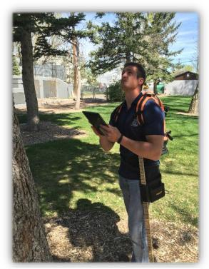
*Figure 3 - Inventorying trees with a tablet and Bluetooth GPS receiver.*
